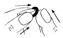
Figure X O-Ring Removal
